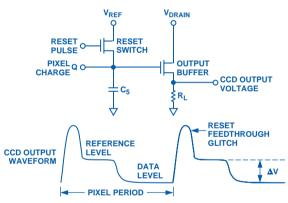
Figure 1. CCD output stage.
