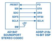
Figure 2. Serial interfacing between digital signal processor and I/O device.
