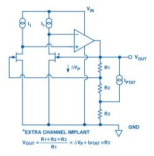
Figure 1. Simplified schematic diagram of ADR29x reference.
