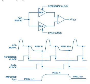
Figure 2. Correlated double sampling. SHA1 samples the reference level, SHA2 the data level. The difference amplifier subtracts the samples, for a measure of the light intensity, reducing common-mode noise.
