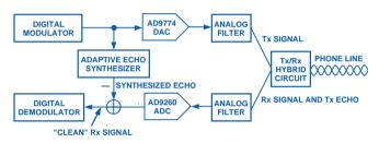
Figure 2. Full-duplex digital error-cancelling modem.
