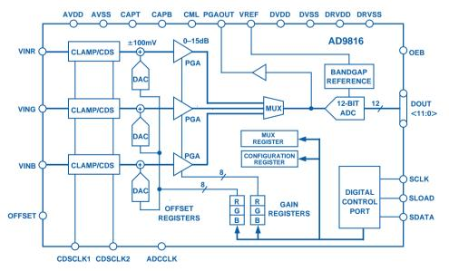
Figure 3. The AD9816 features 3-channel simultaneous sampling, individual per-channel gain and offset adjustment, internal voltage reference, and a 6-MHz, 12-bit A/D converter. The on-board registers are programmed using a 3-wire serial interface.
